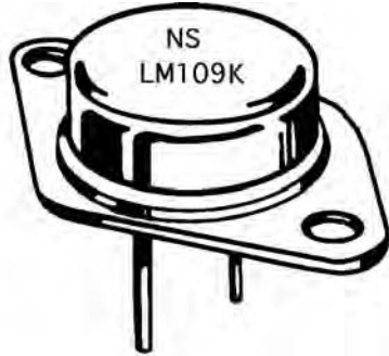
Figure 12.4. National Semiconductor's LM109, designed by the legendary Bob Widlar, and the first 5-volt linear regulator to use a bandgap reference.
