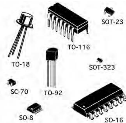
Figure 5.6. Just a few of the packages that have been used for the popular 2N3906, which include metal, plastic, and surface-mount types.
